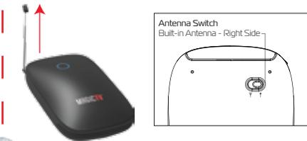
Note: The external antenna is suitable for weak signal areas. Connect the RF cable of the external antenna to the External Antenna Connector. Connect the USB port of the external antenna to the USB Output 5V/1.5A. Slide the antenna switch onto the left side.
